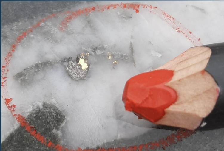
Visible gold from AMD003, which returned 7.5 metres at 55.0g/t Au from 178.1m down hole (ASX AVM 26 September 2025)
